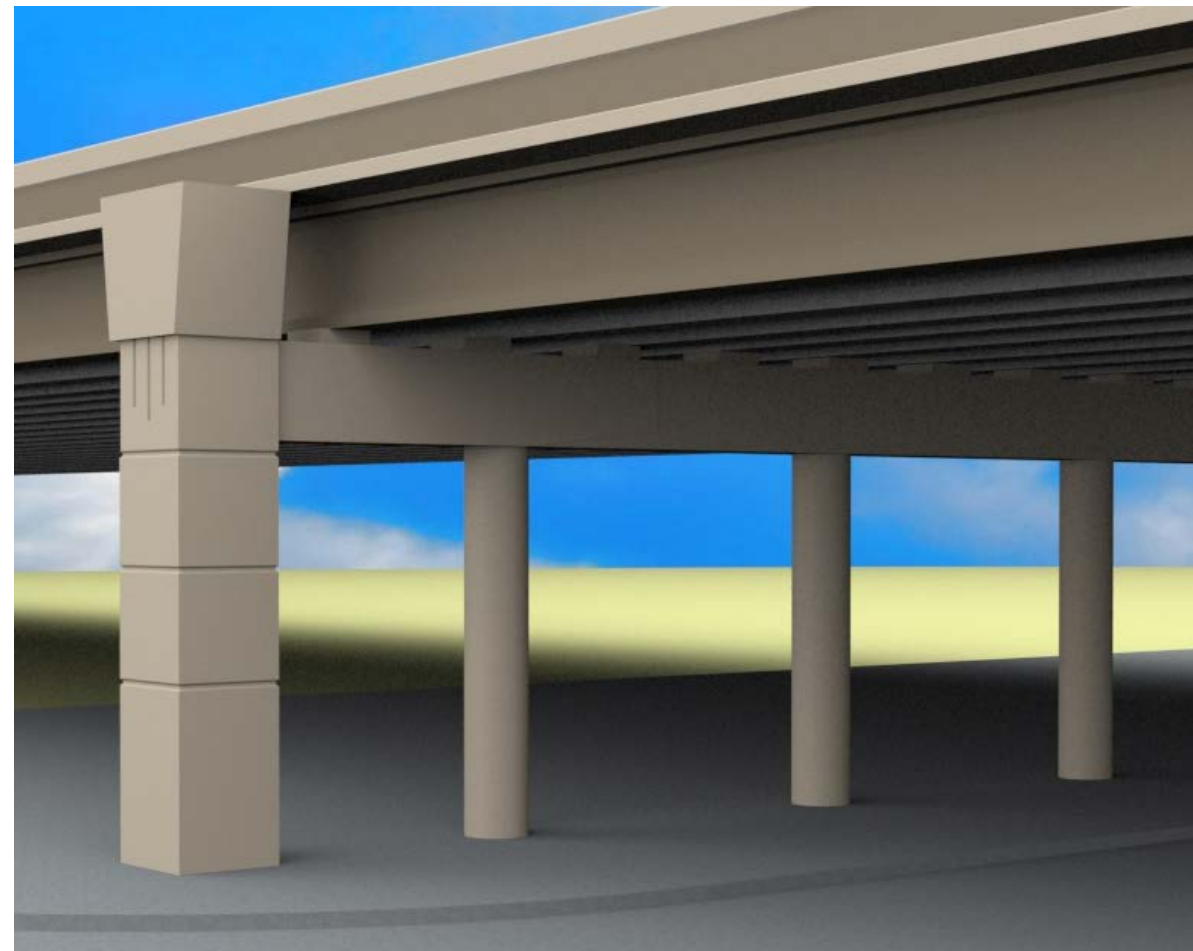
Exterior structural Decorative Column inline with bent where outside widening of structure. Existing interior cylindrical columns remain Decorative column connected to new cap
