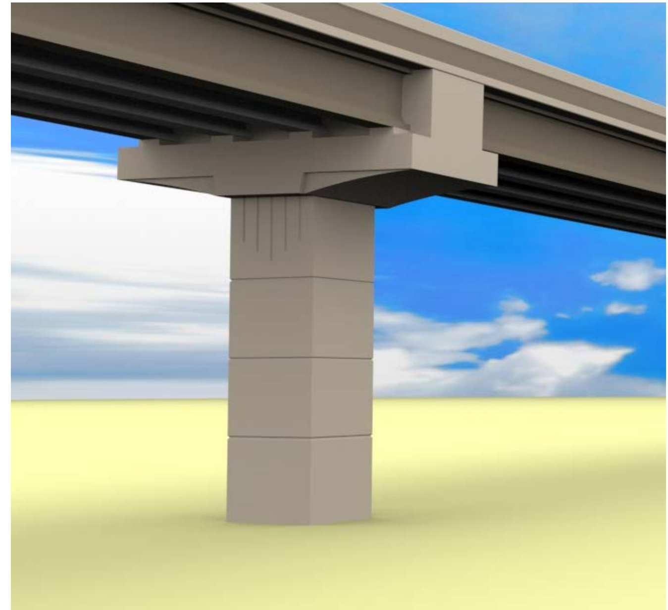
Inverted "T" - Symmetrical Hammer Head – Single Structure
