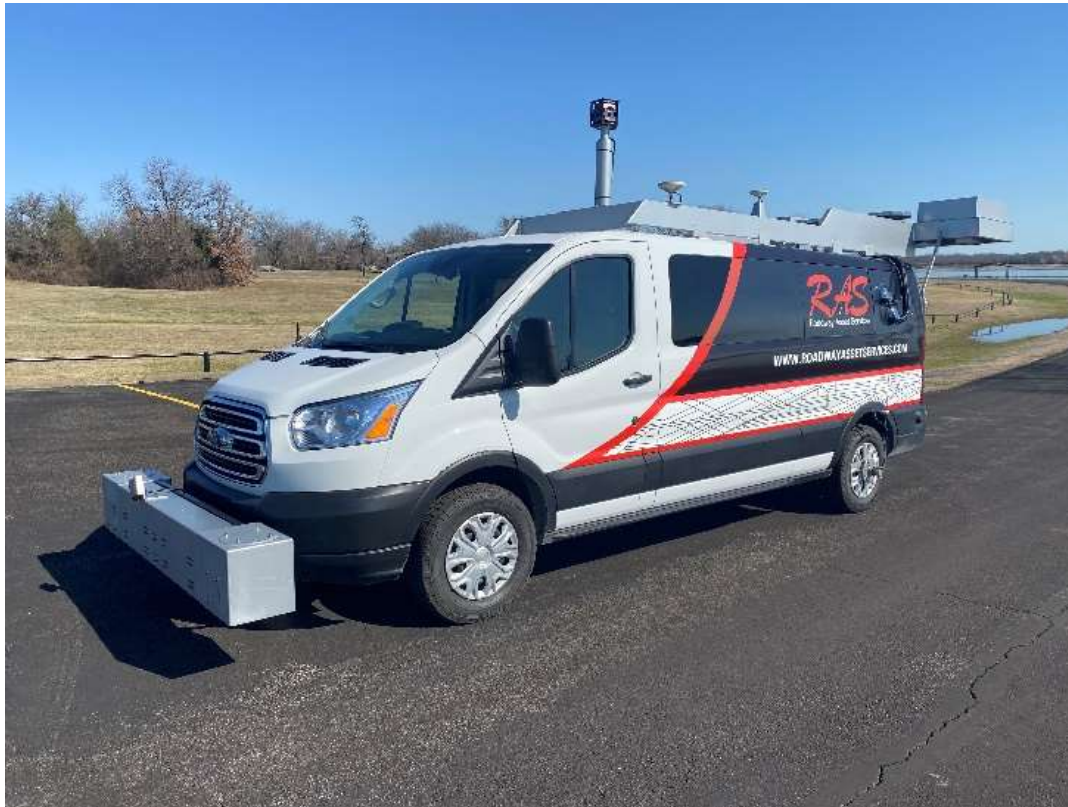
A Roadway Asset Services, LLC automated data collection vehicle
