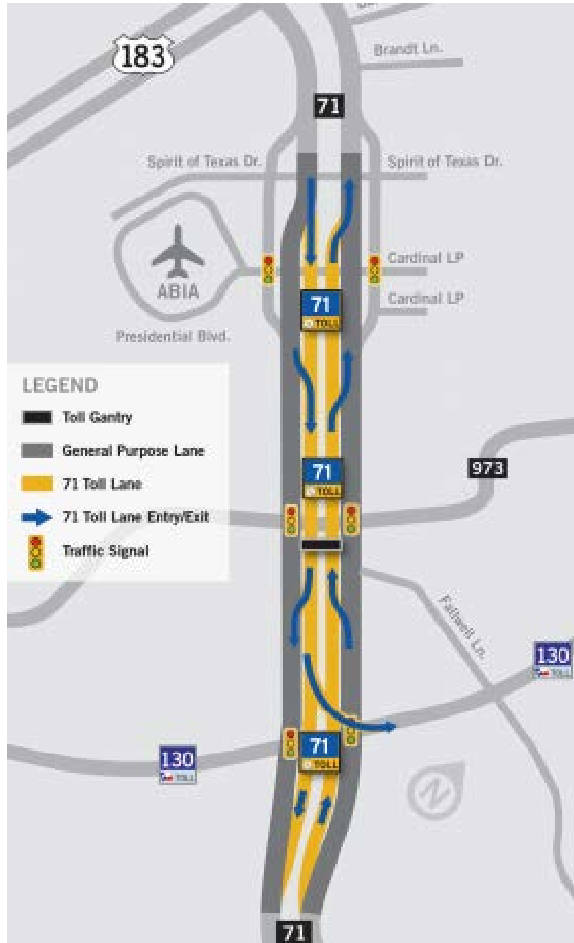
Figure 2-7: 71 Toll Lane Project Configuration
